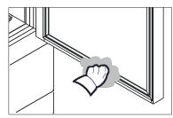
Hand-wash the probe using lukewarm water and a mild detergent or products with biodegradability higher than 90%. Rinse with water and sanitary solution. Do not use detergents containing solvents (such as trichloroethylene, etc) or abrasive powders
