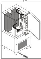
Wash the door gasket with water. Accurately dry with a dry cloth. We recommend wearing protecting gloves throughout the operations.
