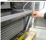
Remove the electrical panel locking screw.
