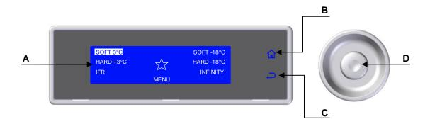
**A–Display**: Displays all the information relative to the menus on the board and the application in progress.
