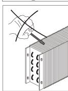
You may clean inside the evaporator after loosening the knobs and rotating the protection component.
